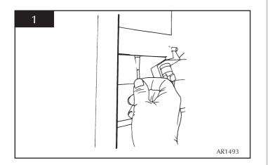
If there are any extractor fans in adjacent rooms, the test must be repeated with the fans running on maximum and interconnecting doors open.
